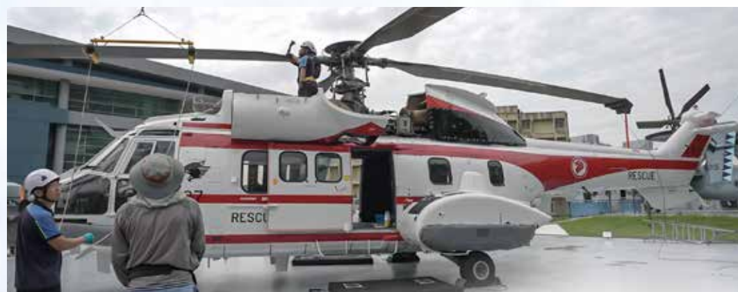
Installation of the helicopter propellers.
